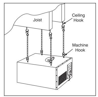
Figure 11. Air filter mounted to the joists.
